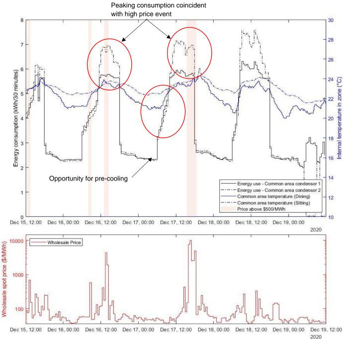
Figure 7.Summer time-series measured data form the Warrigal living laboratory showing energy use for individual condenser units, co-incident internal temperatures for a sample of the zones serviced by these units, and co-incident wholesale spot price during a period with a number of high price events.
