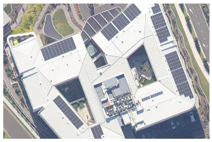
Figure 5 - Aerial view of the living laboratory with the 99 kWp PV system and HVAC service on the roof.
