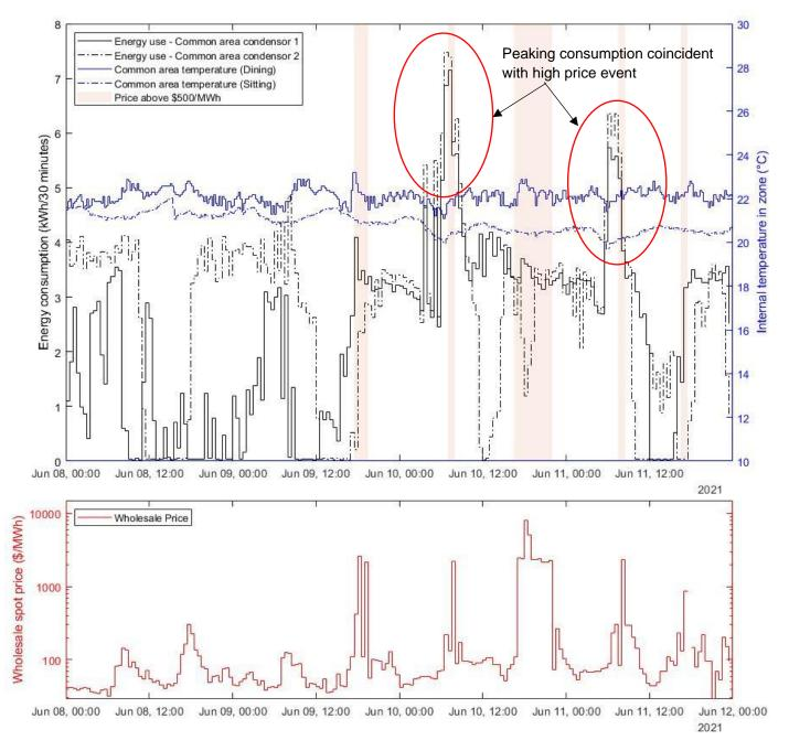
Figure 8. Winter time-series measured data form the Warrigal living laboratory showing energy use for individual condenser units, co-incident internal temperatures for a sample of the zones serviced by these units, and co-incident wholesale spot price during a period with a number of high price events.
