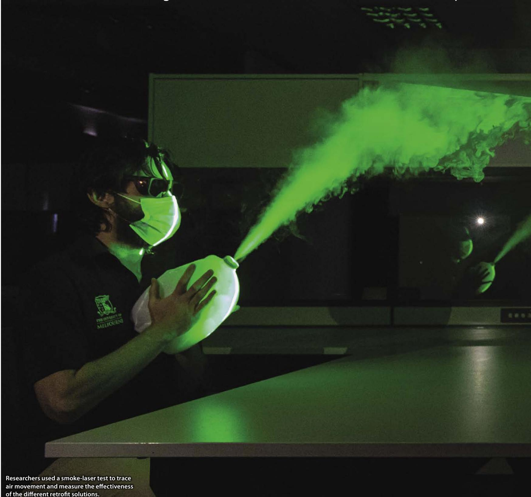
Researchers used a smoke-laser test to trace air movement and measure the effectiveness of the different retrofit solutions.
