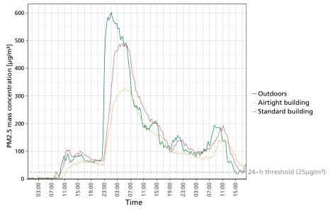
Figure 2: Performance of airtight and standard buildings during smoke event
