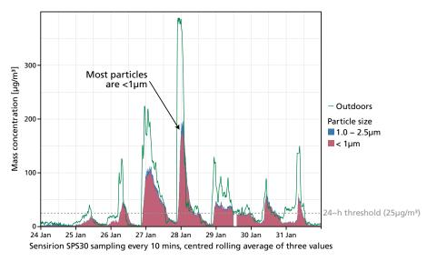
Figure 3: Smoke infiltration in an extremely airtight building
