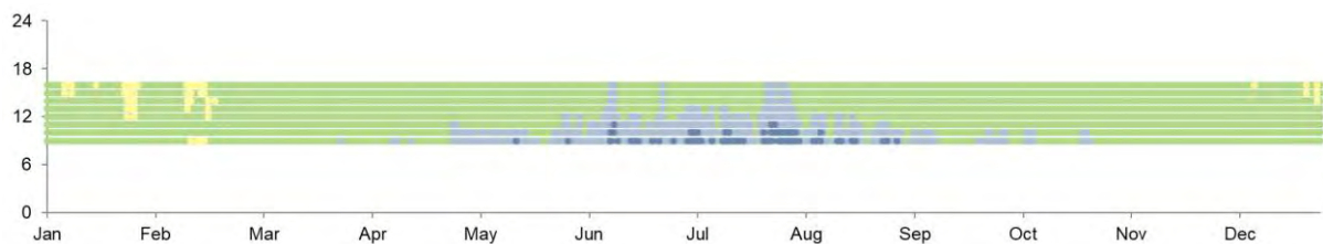
Figure 8. Heatmap of operating hours: Addition of evaporative cooling to the passive cooling system at 24°C ground temperature case
